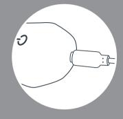
**3.** The cable will magnetically attach itself into place. The power button LED will pulsate slowly to indicate charging.
