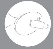
3. The cable will magnetically attach into place. The power button LED light will pulsate slowly to indicate charging.
