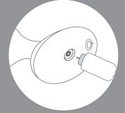
2. Line up the magnetic charging head with the charging contact.
