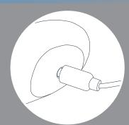
3. The cable will magnetically attach itself into place. The power button LED light will pulsate slowly to indicate charging.
