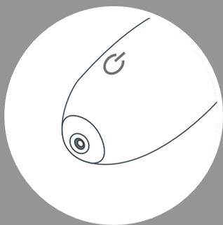
1. The charging contact is a small metal circle located at the bottom of the device.
