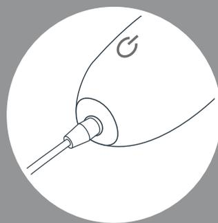
3. The cable will magnetically attach itself into place. The power button LED will pulsate slowly to indicate charging.
