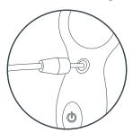
Insert the charging pin through the rubber into the port. The rubber will stretch open to accomodate the pin. It's a tight fit!
